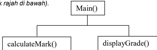
Function **main()** will ask user to read carry mark and final mark (valid value for carry mark and final mark is between range 0 to 50). Both of the value will be sent to **calculateMark()** where inside this function both of the value will be add and statement passed will be display if the total mark is more or equal than 60 or else it will display failed. Function **calculateMark()** will return total mark.
